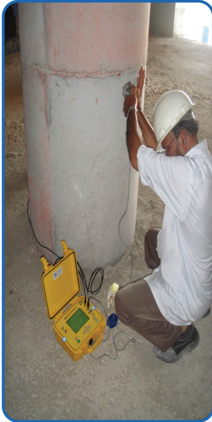
Concrete column Sismo test tool to test the strength of the column for longevity and sturdiness against the elements.
